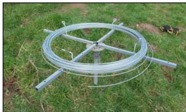
fence. You have a nice straight line of wire, ready to be attached to the posts. Without the Spinning Jenny the wire will probably form loops and be difficult or even impossible to pull straight. I made this one ready for the spring, as that's when I normally do that kind of work. It's a really good tool to have in your shed.
